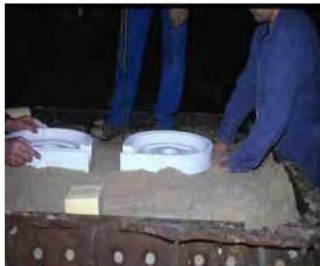
\* Fig 7 – Sand compaction with two carousel filters
