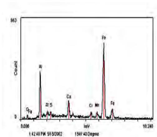
\*Figure 9 – EDS Analysis of oxide inclusions
