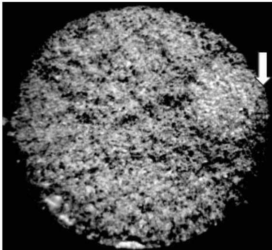
**Figure 4: fracture surface of a tensile test specimen. The arrow points the location at which a water impregnated hyssop has been put in contact with the sample surface. Note the approximately round, bright area of about 1.5 mm diameter that originates from the contact point. Total sample diameter is 6.5mm.**
