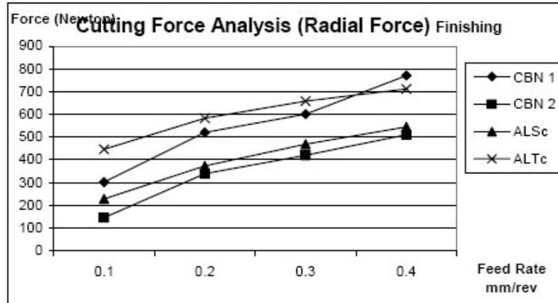
Figure 11 cutting forces results for Finishing operation
