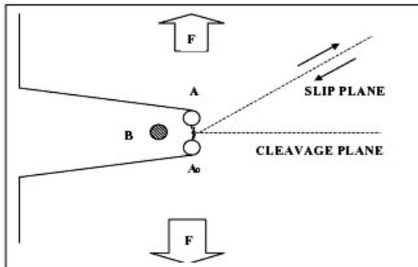
**Figure 7: schematic representation of the weakening of A-A atom bonds at a surface crack tip as a result of the interaction with an atom or molecule B supplied by the surrounding liquid.**
