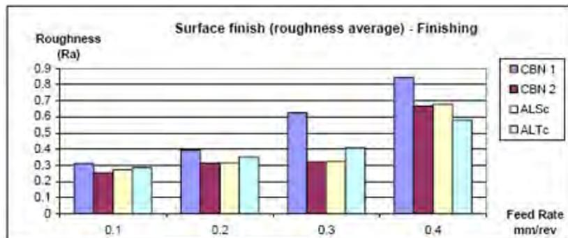
Figure 13 Surface Finish results for Finishing operation
