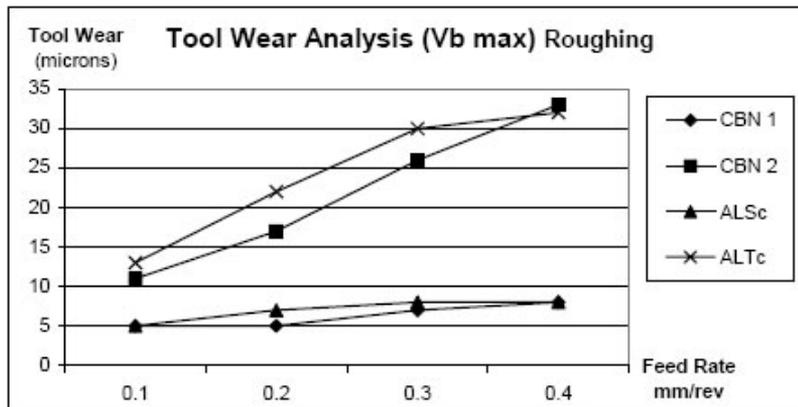
**Figure 8 Tool wear results for Roughing operation**
