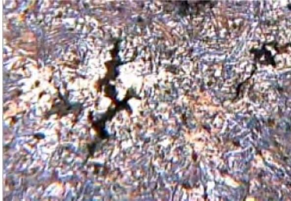
**Figure 3: Typical cracking of LTF regions of ADI samples after plastic deformation.**
