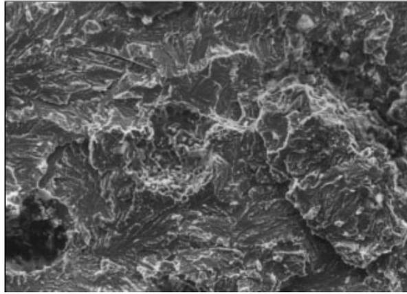
**Figure 5: Fracture surface of ADI embrittled by water (500x).**
