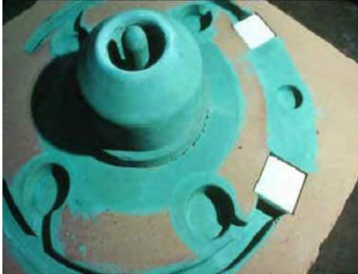
\*Fig 5 – Horizontal implementation of Reticulated Ceramic Filters
