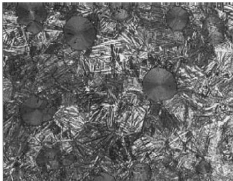
**Figure 3 – microstructure of ADI presenting a common ausferritic matrix of ADI casting grade 1 (500 X)**
