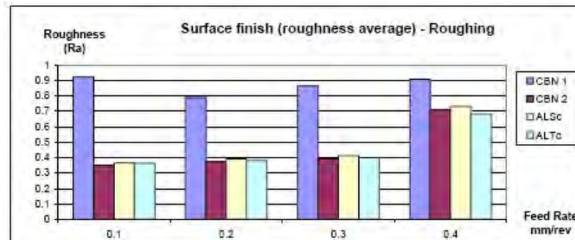
Figure 12 Surface Finish results for Roughing operation
