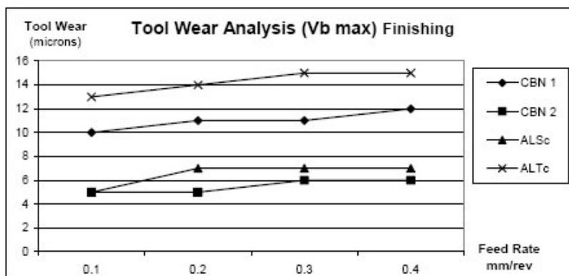
**Figure 9 Tool wear results for Finishing operation**
