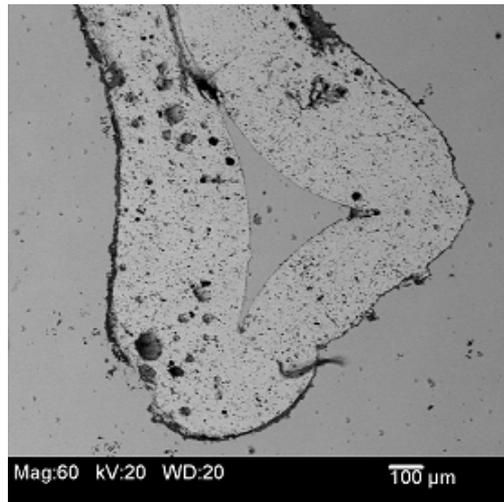
\*Figure 8 – Electron Microscope Photo of Ceramic Filter material with oxide inclusions sintered on
