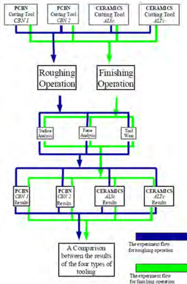
**Figure 4 – The experiment design flowchart**
