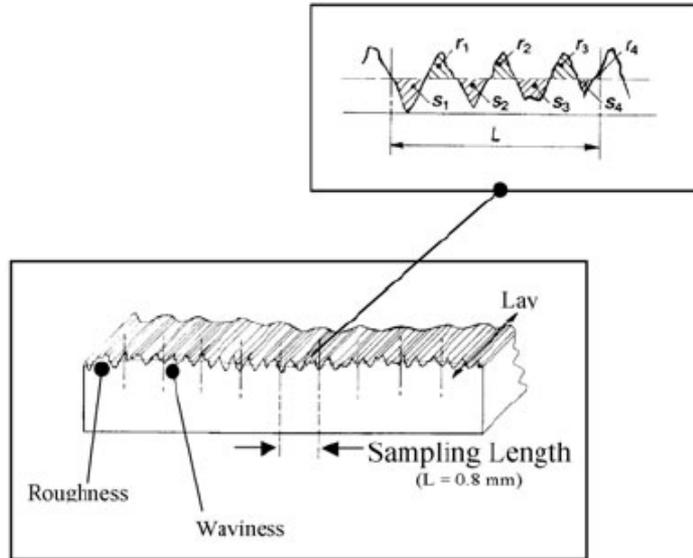
**Figure 6 - the fundamental parameters of surface texture [13]**
