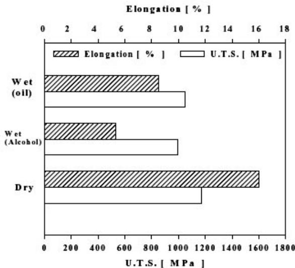
**Figure 2: Change of UTS and elongation caused by contact with lubricant oil and isopropyl alcohol.**
