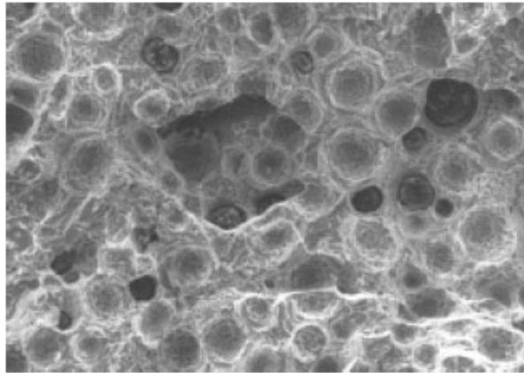
**Figure 6: Predominantly ductile fracture surface of ADI broke in contact with water, shown at a location far from the fracture initiation site (200x).**
