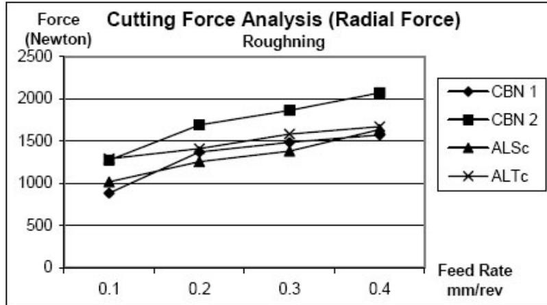
Figure 10 cutting forces results for Roughing operation
