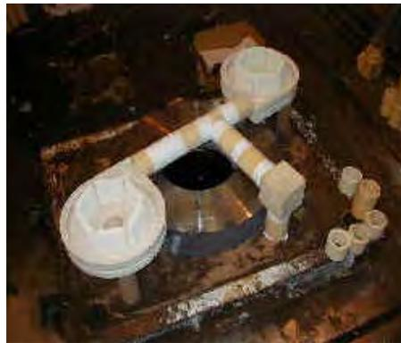
\*Fig 6 – Attachment of carousel filters
