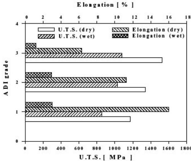
**Figure 1: Change in UTS and elongation as a result of tensile testing of ADI grades 1, 2 and 3 in contact with water.**
