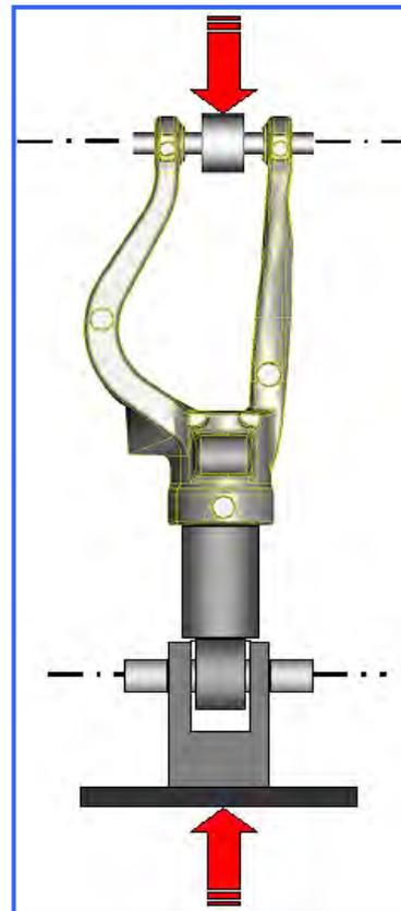
**Figure 5 : Fatigue testing of the suspension fork**
