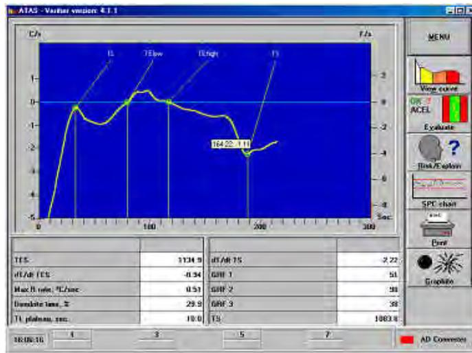
**Items to note:** Very erratic cooling, shown here by the 1st derivative curve. Graphite Factor 1 (GRF1) is low, indicating a low amount of eutectic graphite and Graphite Factor 2 (GRF2) is high, which is a measurement of the angle at the solidus on the 1st derivative curve. These two factors are an indication that the nucleation status of the iron is poor, which will lead to a lower nodularity and nodule count with an increased risk for shrinkage defects.
