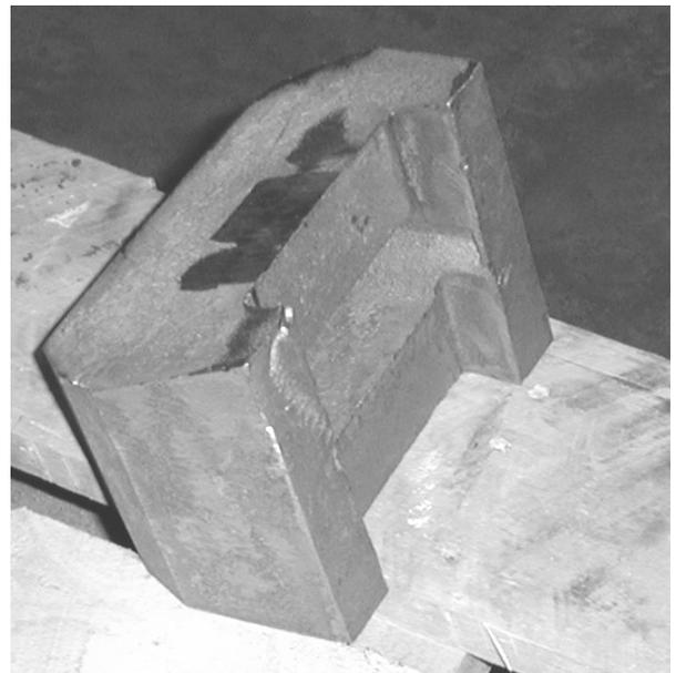
**Figure 19: Mulching Hammer**
