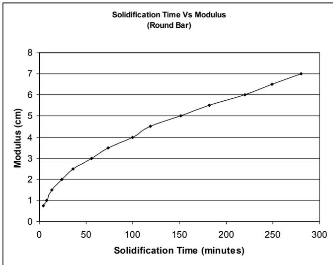
**Figure 10 : Solidification Time vs Modulus.**
