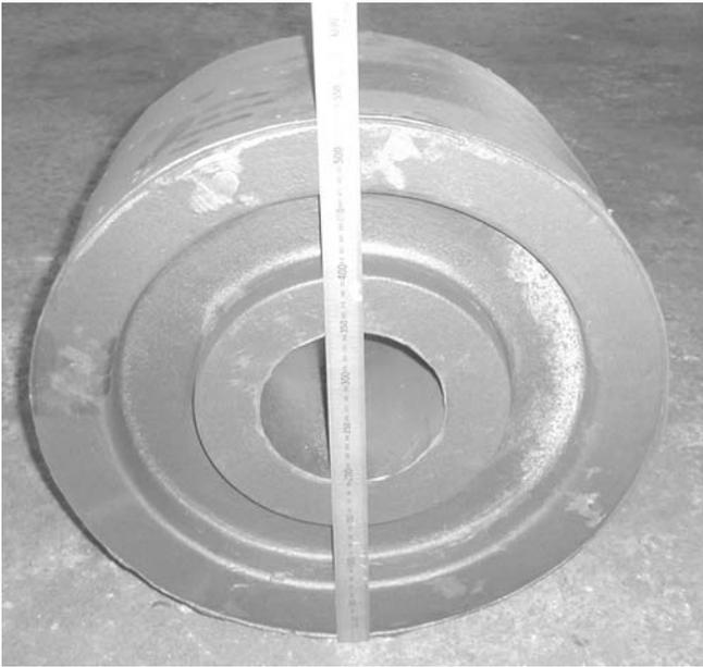
**Figure 16 : Roller Casting – 530mm dia x 300mm high**
