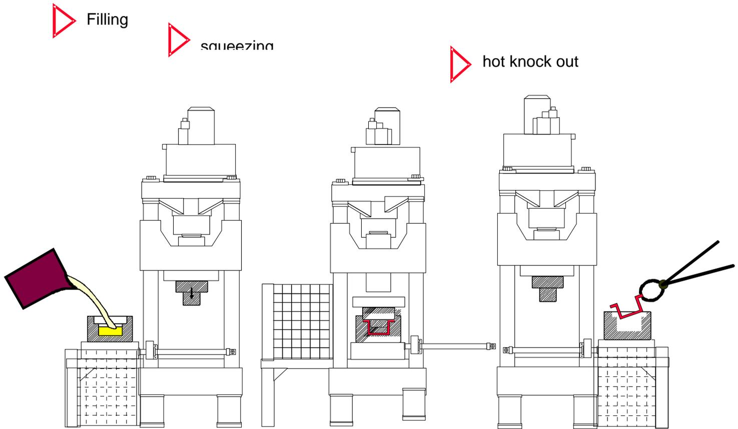
**Figure 2 : Squeeze casting process**
