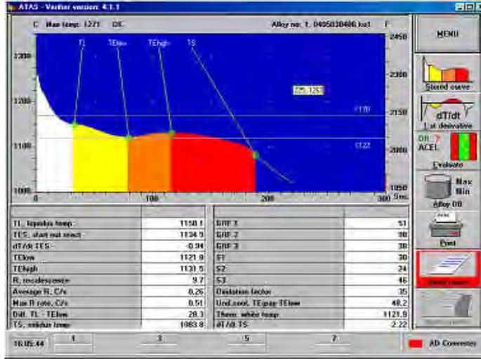
**Items to note:** Large yellow area (S1) which indicates a large amount of primary austenite. This is a critical measurement to show macroshrinkage tendency. The more primary austenite, the larger the dendritic growth making feeding with risers more difficult.
