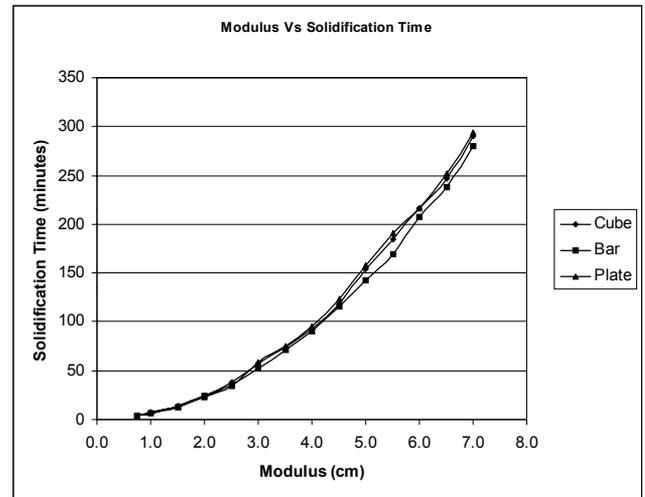
**Figure 8 : Modulus vs Calculated Solidification Time**
