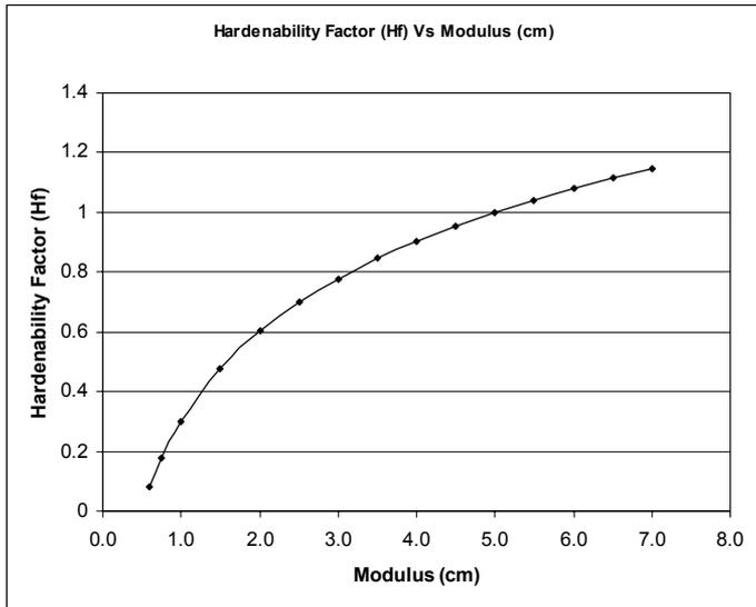
**Figure 14 : Modulus vs Hardenability Factor**
