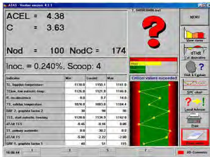
ATAS screen showing the iron's solidifications characteristics are not within limits set by Neenah Foundry.
