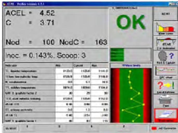
ATAS screen showing all the parameters fall within Neenah Foundry limits and it is OK to pour industrial castings.
