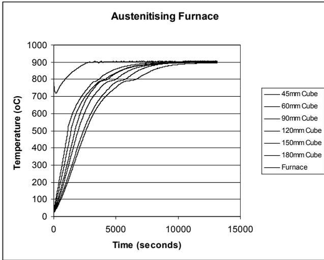
**Figure 2 : Heating to 900°C ( Time vs Temperature °C )**
