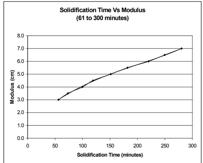
**Figure 12 : Solidification Time vs Modulus ( 61 to 300 minutes )**
