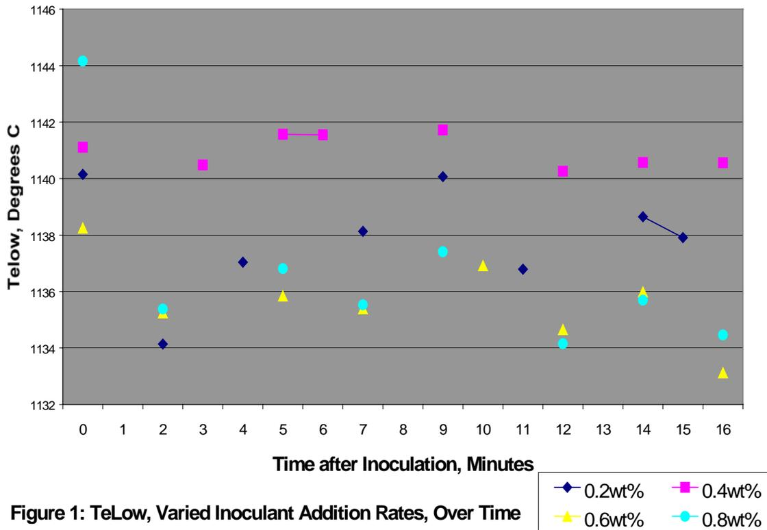
Figure 1: TeLow, Varied Inoculant Addition Rates, Over Time
