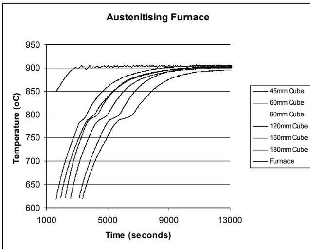
**Figure 3: Arrest at Upper Critical Temperature**
