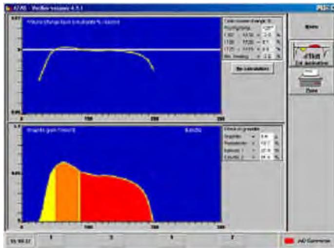
**Items to note:** Much smoother graphite precipitation. The Eutectic 2 value is much higher 55, showing 55% of the graphite precipitated is late stage. This will give a much higher nodule count and help offset microshrink.
