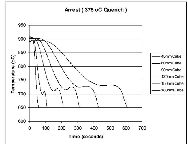
**Figure 5 : Arrest during Salt Quench**
