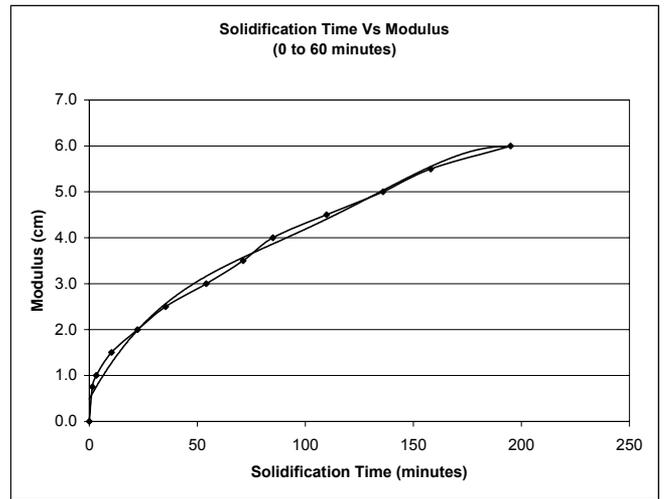
**Figure 11 : Solidification Time vs Modulus ( 0 to 60 minutes )**
