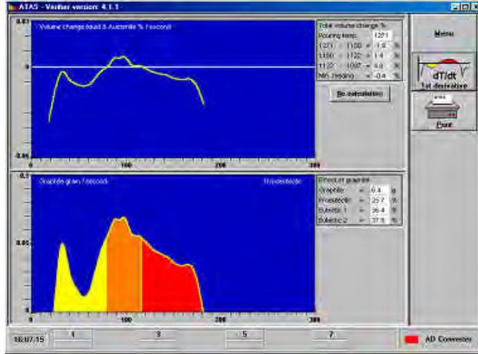
**Items to note:** Very erratic graphite precipitation. The eutectic two value is quite low, 37.8, indicating that only 37% of the graphite is coming out in the last stages of solidification to help offset microshrink that occurs at the end of solidification. This eutectic two measurement can be used as another measurement of metallurgical conditions, a higher value is desirable.
