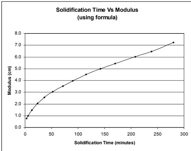
**Figure 13 : Solidification Time vs Modulus (using combined formula)**
