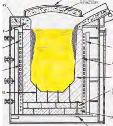
*Figure 1: Typical slag buildup in a coreless induction furnace (gray shaded areas)*
