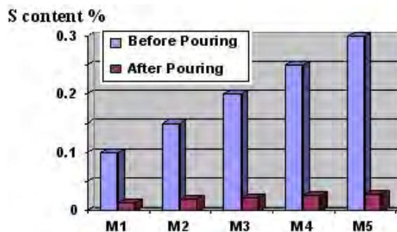
*Figure 7 - Sulfur % content of furan bonded sand.*
