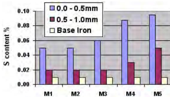
Figure 9 - Sulfur % level of Casting
