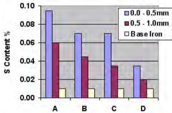
*Figure 6 - Sulfur % content of casting at different sections*
