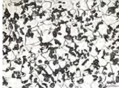
Fig. 2. Microstructure of an as-sprayformed eutectoid iron, nital etched.
