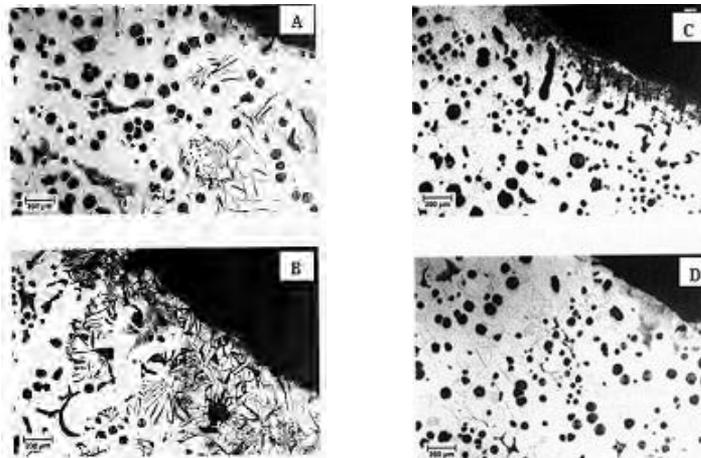
**Figure 4 - Casting structures using Coatings A,B,C & D**
