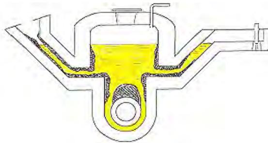
**Figure 4: Traditional throated pressure pour vessel showing slag buildup in (gray shaded areas)**
