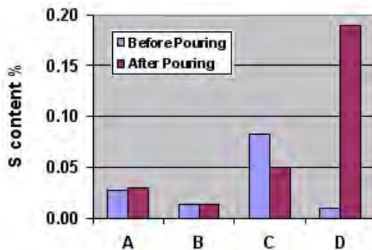
**Figure 5 - Sulfur % content of Coating samples before and after pouring**
