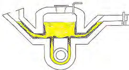
**Figure 5: Throatless pressure pour vessel showing slag buildup in (gray shaded areas)**
