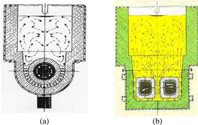
**Figure 3: Circulation and metal flow (shown by the arrows) in a (3a) single loop inductor and (3b) double loop inductor.**
