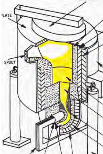
**Figure 2: Slag buildup in the inductor and throat of a vertical channel furnace (gray shaded area)**
