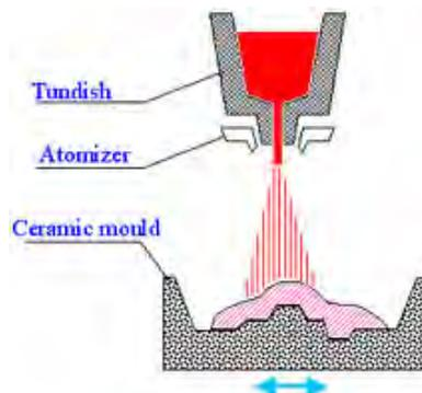
Fig. 1. Principle of sprayforming technology
