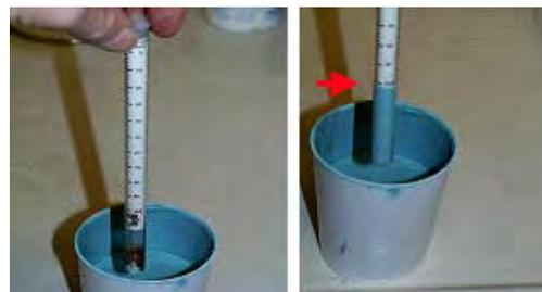
*Figure 3 - Measurement of viscosity with a Baume Stick*
