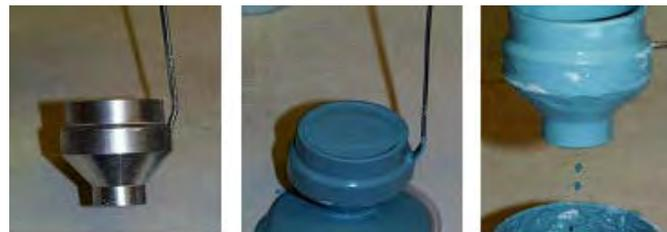
*Figure 2 - Measurement of viscosity with a Flow Cup*
