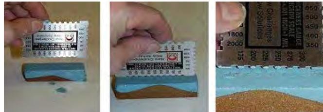
*Figure 1 - Measuring the wet thickness layer of a coating*
