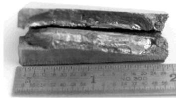
b. Cross section of defect
