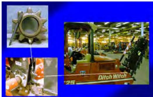
**Figure 3 -** ADI gear in trenching Equipment. (Courtesy of Farrar Corporation)
