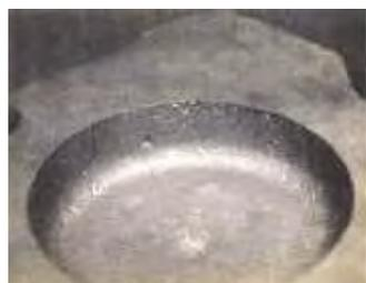
*a: Wrinkles on automotive brake caliper*
