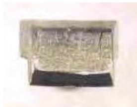
*d: Surface wrinkles on pulley hub*
