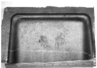
*e: Surface wrinkles in oil pan which leaked*
