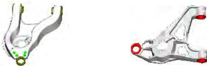
**Figure 4 -** The stamped steel welded (left view) and the ADI (right view) lower control arms for a heavy duty Dodge Ram pickup truck. (Courtesy of Intermet Corporation and Daimler Chrysler Corporation.)
