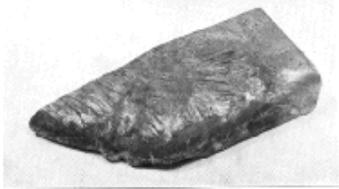
Figure 7: Severe surface wrinkling resulting from solidification against accumulations of lustrous carbon.
