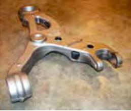
controlled volume fraction of carbide present was also discussed for its growing interest for agricultural applications. This material shows improved wear performance over ADI along with impact properties that can be several times that of abrasion resistant irons. Figure 6 shows a CADI plow point that has been in production since the early 1990's.
