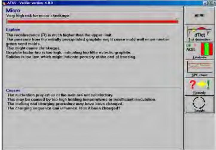
Pic. 3. This screen shows how the expert system has interpreted the thermal data.
