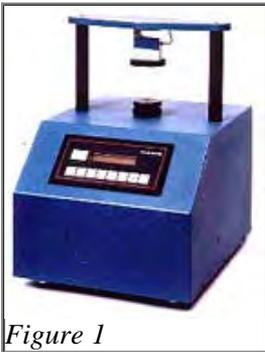
Modern strength machines utilize load cells for measuring sand strength characteristics, and modern permeters use new air flow technology for measuring permeability. In addition, these modern devices provide digital readouts of the data and allow exportation of the data to PC computers so that trends can be identified more quickly, leading to better control.
