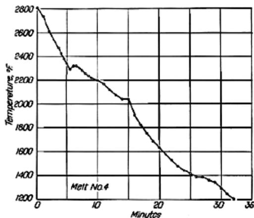
Figure 1 - Cooling curve of Melt No. 4
