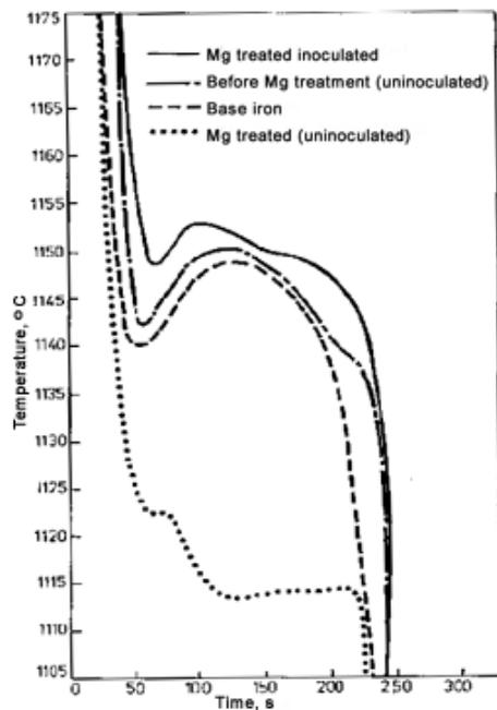
Figure 17 - TA Curves at each stage of a Fischer process Ductile Iron
