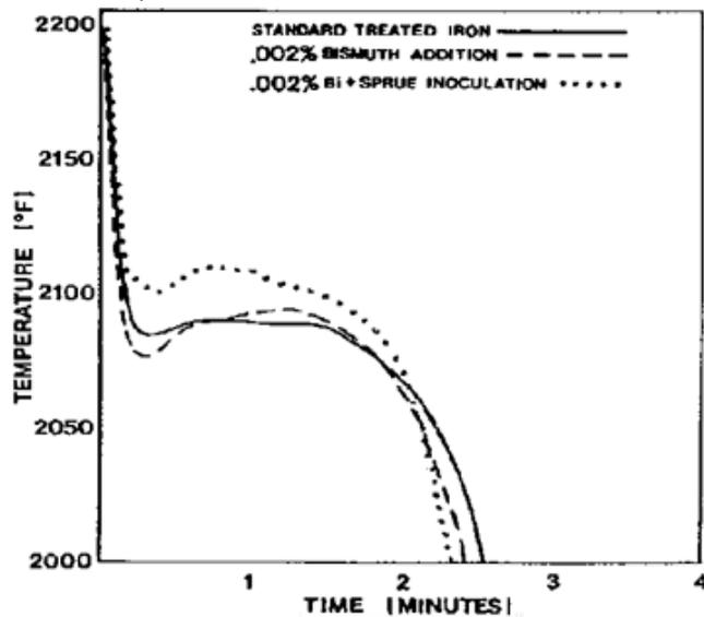
Figure 15 - Standard treated iron vs. bismuth and bismuth and sprue inoculation.
