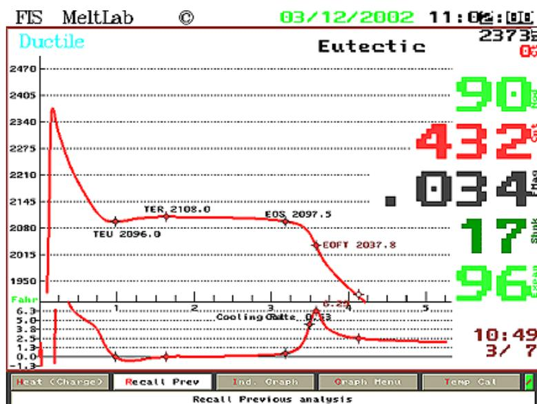
The inoculant sharply reduced the shrinkage potential and changed the solidification mode to eutectic. Where in the pouring furnace iron, the bulk of solidification occurred between 2040.0 and 2040.3, here the solidification is occurring between 2096.0 and 2108.0, a major change of over 60 degrees higher.
