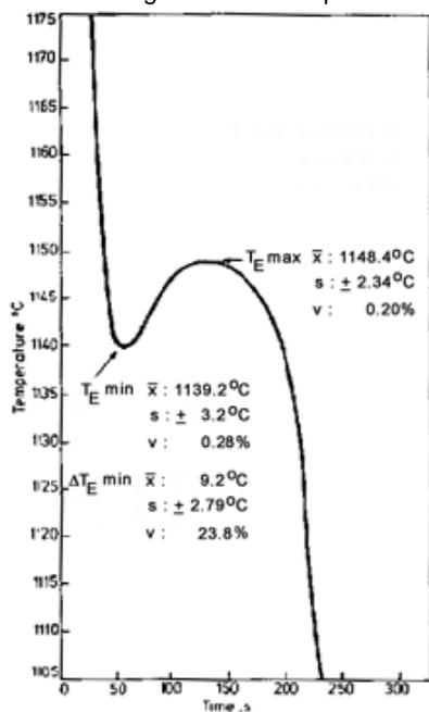
Figure 18 - Cooling curve of a composition adjusted base iron.
