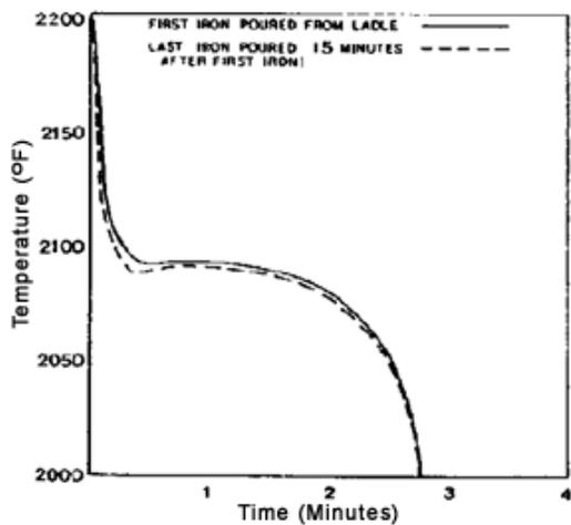
Figure 14 - Initial iron poured vs. last iron five minutes later.
