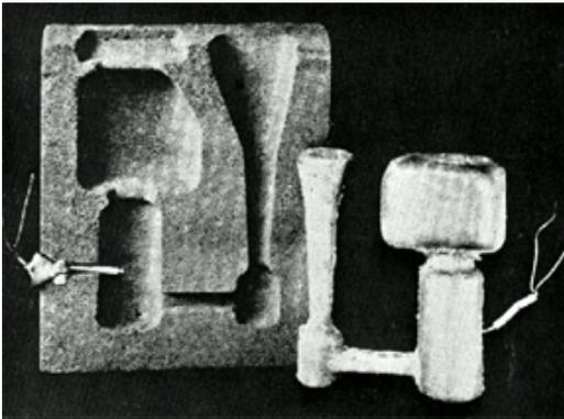
**Figure 6** - Core mold and test casting.
