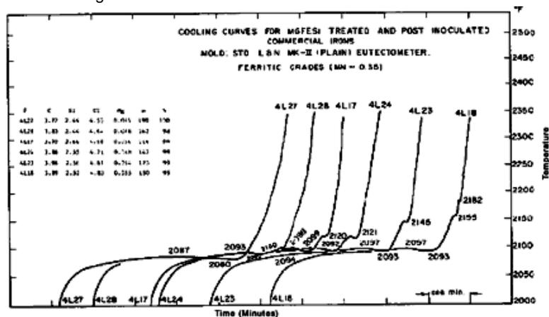
Figure 2 - Cooling curves of castings made from Iron No. 133. Curves on left from castings poured 2 minutes after inoculation. Curves on right from castings poured 32 minutes after inoculation.
