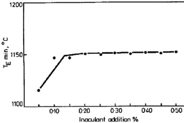
**Figure 23** - Method used to establish the optimum necessary inoculant level.
