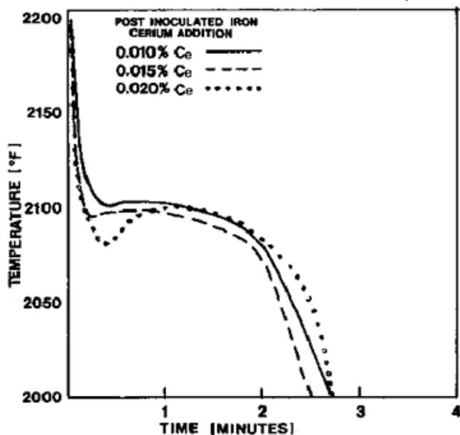
Figure 16 - Effect of increasing cerium in MG treatment on inoculated iron cooling curve.
