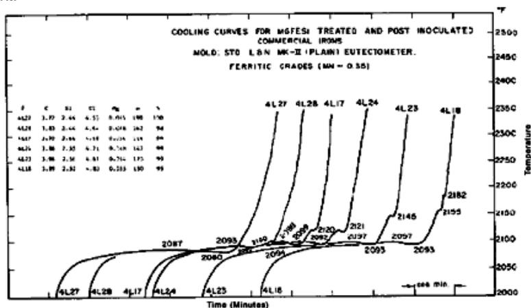
**Figure 12** - Cooling curves for MgFeSi treated and post inoculated commercial
