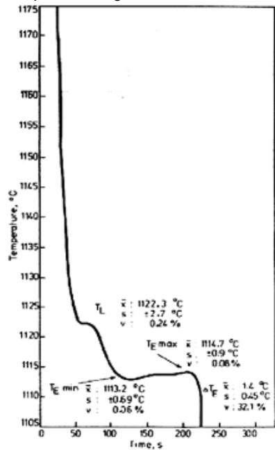
Figure 20 - Cooling-curve for an uninoculated magnesium-treated melt.
