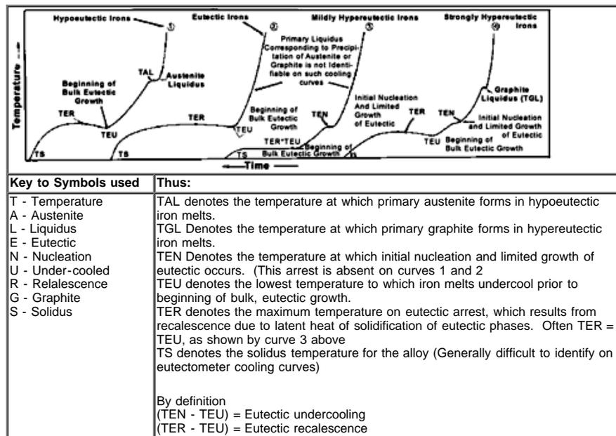
**Figure 11** - Typical eutectometer cooling curves illustrating the nomenclature used in text.
