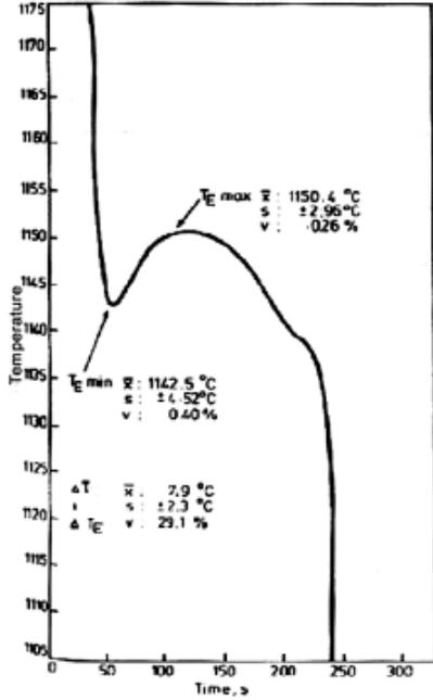
Figure 19 - Cooling curve prior to magnesium treatment in the Fischer converter.
