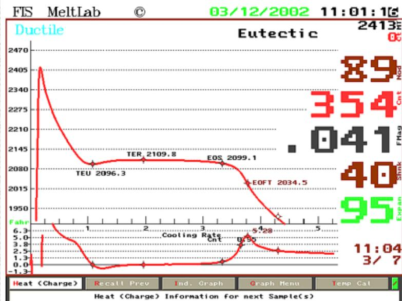
Here the bulk of solidification occurred between 2096.3 and 2109.8 degrees. This is extremely close to the previous trial of 2096.0 and 2108.0, with the difference in the higher number reflecting more effective magnesium.
