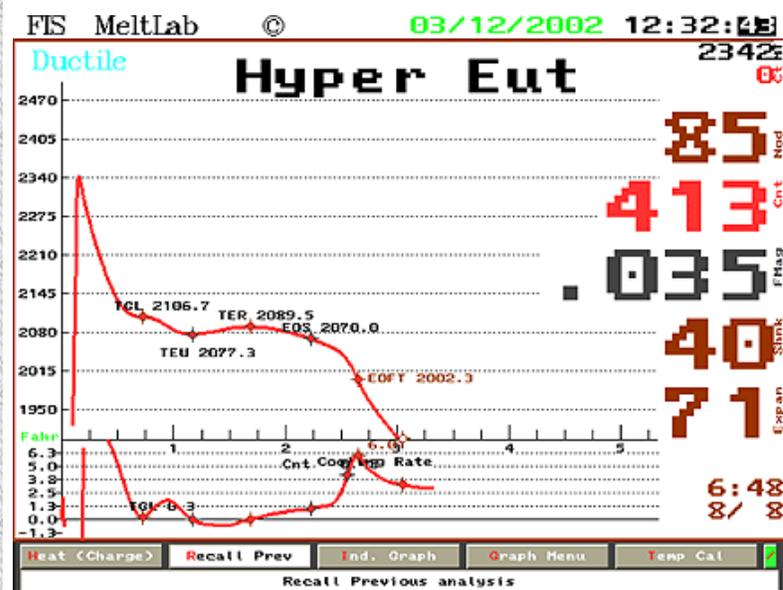
This is an example of new shrinkage and expansion values. This sample shows low expansion and moderate shrinkage potential, possibly due to hypereutectic arrest.
