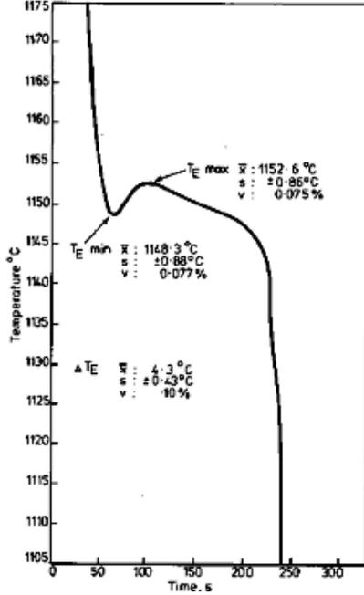
**Figure 21** - Cooling curve of treated inoculated iron taken from the ladle just prior to pouring.
