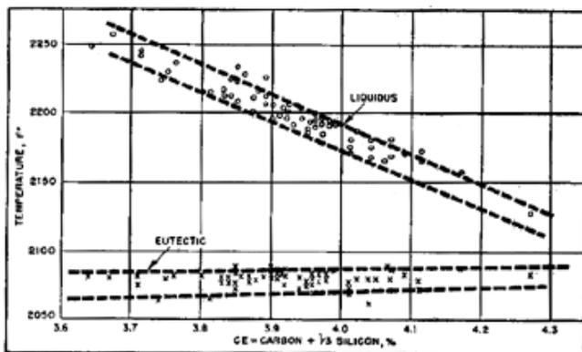
**Figure 3** - Relationship is shown between liquidus and eutectic thermal arrest temperatures and carbon equivalent determined by chemical analysis.
