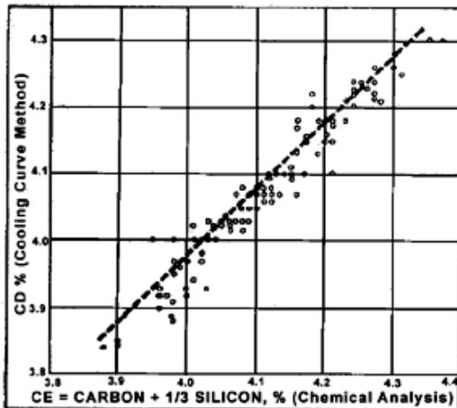
**Figure 4** - Relationship of carbon equivalent data determined by cooling curve method and by chemical analysis.
