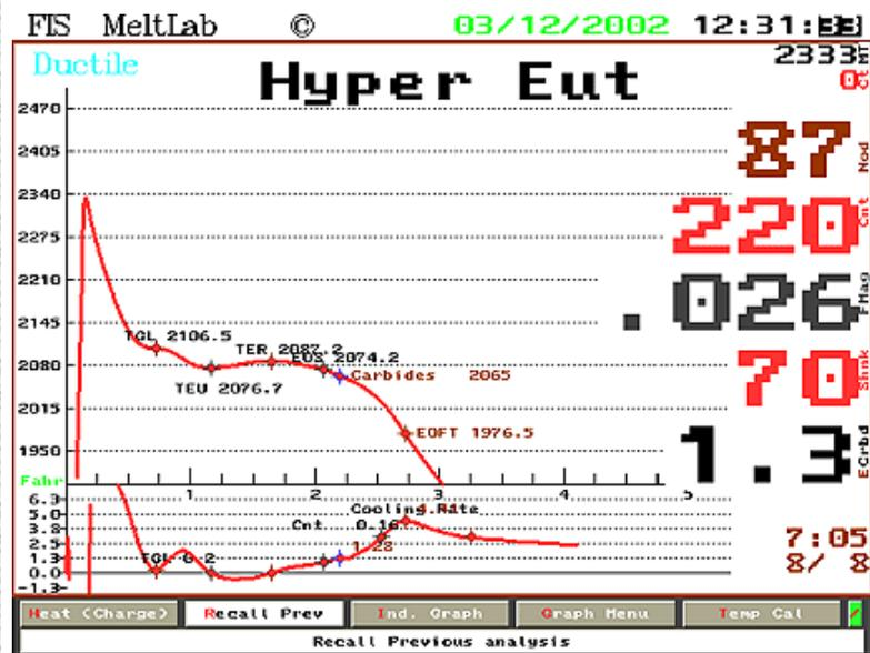
This is an example of an iron with very low graphite expansion that resulted in actual carbide formation. Due to the low magnesium, this could have been carbides in d or e-flake. Note how the rate of cooling rises at the end of the eutectic reaction. This iron was not from the same foundry, and was inoculated with only ferro-silicon.
