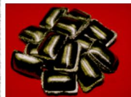
Nodu-Bloc briquettes have an almond shape and measure 1.25 inch by 1.0 inch by 1/2 inch, each having a volume of approximately 5 cubic centimeters (see **Figure 7**). Recently, a somewhat larger pressed disc measuring 4.75 inches in diameter and 1.25 inch thick (350 cc's) and containing either
