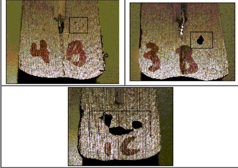
*Figure 1. These are three examples of different levels of macro-shrinkage in thermal analysis cups. Shrinkage occurs at the point of the last metal to solidify, so is located around the thermal couple for easy detection. Some suck-in occurred in the first and second sample.*
