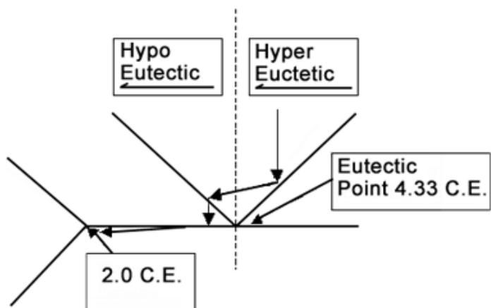
Figure 8. Expanded region of eutectic zone due to magnesium suppression of graphite formation.
