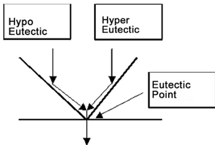
Figure 2. Phase diagram showing movement of carbon concentration in liquid metal as iron solidifies.
