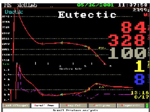
Figure 7. Single arrest eutectic mode solidification
