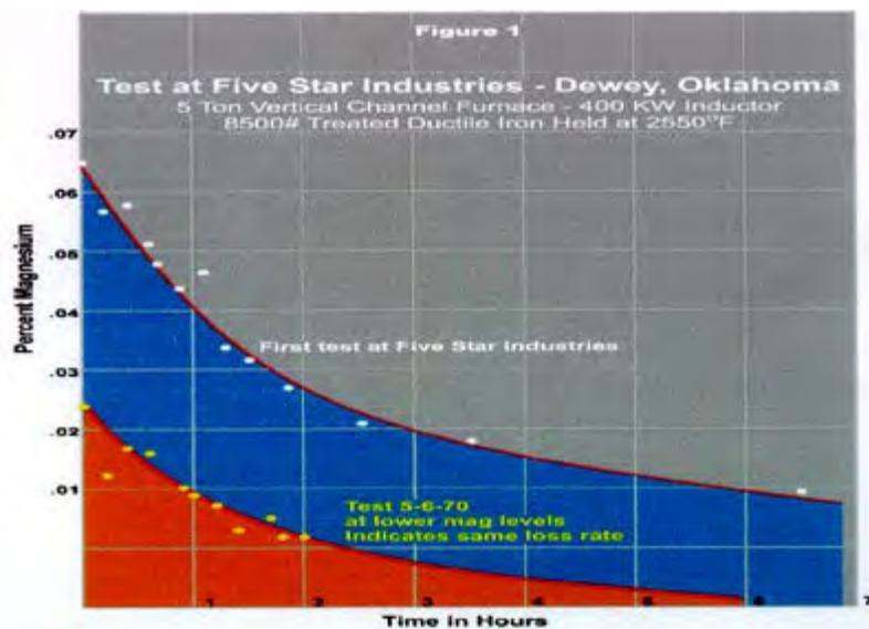
**Figure 1 - Magnesium Fade Rate vs. Magnesium Level (Note higher level indicates higher fade rate)**
