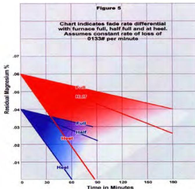
**Figure 4 - Magnesium Fade Rates at Differing Furnace Levels**
