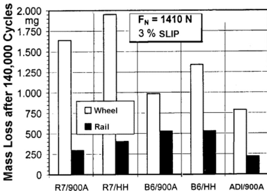
Figure 3- Mass loss for various wheel/rail material combinations at 3% slip and  $F_N = 1410 \text{ N}$
