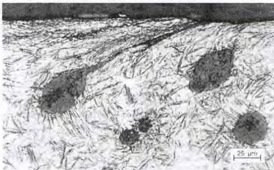
**Figure 7- Surface microstructure of the ADI test sample after roll / slip testing at  $F_N=3935$  N**
