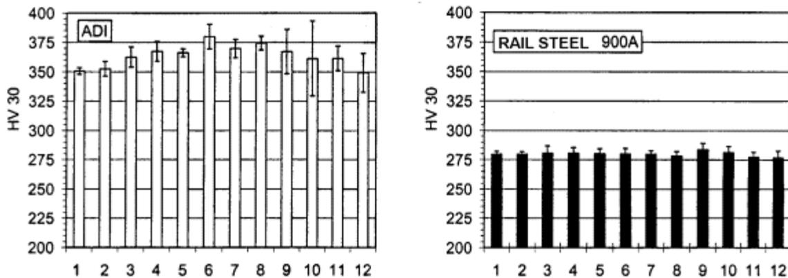
Figure 2- Microhardness traverse data for ADI and 900A Rail Steel
