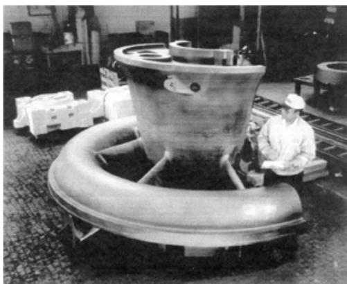
*Here's an example of a 40.3 type casting - an inlet housing (26,956 pounds)*
