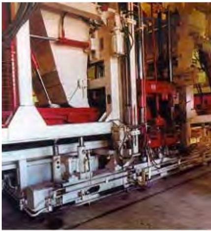
Figure 1: A paver machine that is used to briquette alloys for the foundry industry.
