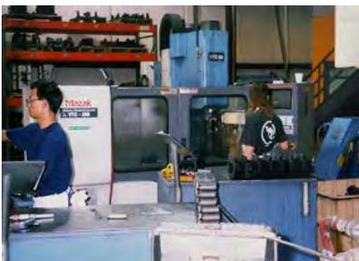
BCI offers machining service in house using one Mazak HTC-400 Horizontal Machining Center and one Mazak VTC-20B Vertical Machining Center. Also available is on Wesel Knee Mill LC-1850vs. This equipment provides a full range of capabilities.
