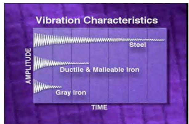
processing costs, the possible elimination in heat treat, improved vibration damping properties and the domestic availability of ductile iron bars and castings.
