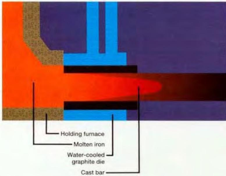
The heat from the molten iron core reheats the outer skin that was rapidly chilled inside the die. The matrix in the rim is transformed to austenite and cools in still air as the bar moves horizontally along a series of rollers. The center of the bar is allowed to solidify and cool in still air. The resulting microstructure in the continuous cast bar is a homogenized matrix of pearlite, ferrite, or a ratio of the two, depending on the grade being produced.
