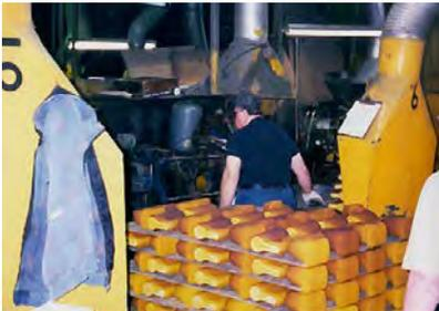
Beginning the casting process in the molding department, the foundry utilizes green sand molding equipment with five 14x19 Hunter Automatics, one 20x24 Hunter Automatic and one 20x26 Roberts Sinto Automatic.
