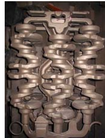
Image 6: same crankshaft cluster redesigned after lanthanum addition. 6 crankshafts are placed within the same volume.
