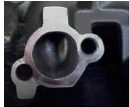
Image 12 : Exhaust Manifold (flange view)
