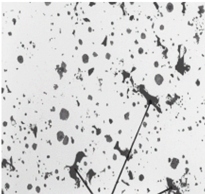
Image 3: SG iron structure without La showing micro-shrinkages
