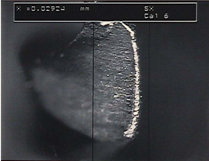
Figure 3 : Low magnification image of a drill land with the wear profile shown.
