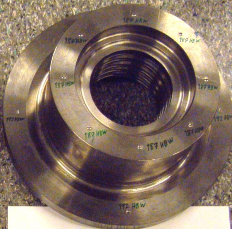
Swivel housing for Rotator IR 10; 36 kg casting in
