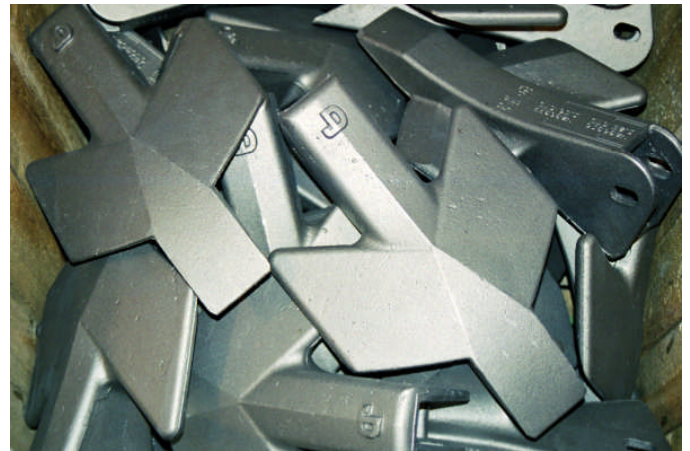
Figure 19- John Deere LaserRip™ CADI ripper points. (Courtesy of John Deere and ThyssenKrupp Waupaca)
