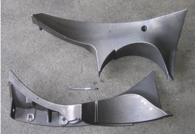
Figure 10- An ADI Grain Deflector for a harvesting combine.
