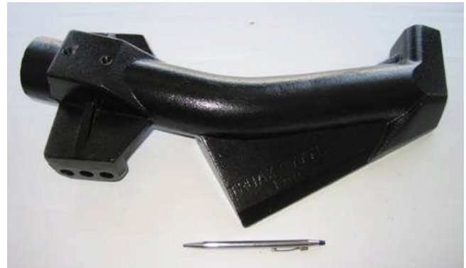
Figure 4a shows a seed boot constructed of welded steel. Figure 4b shows the ADI casting that replaced it as a cost and weight reduction. (Courtesy of Smith Foundry).
