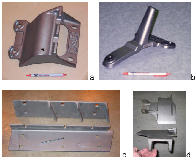
Figure 20 shows several CADI harvester applications. a) bucket, b) thrashing tine, c) flight, d) scraper blade.
