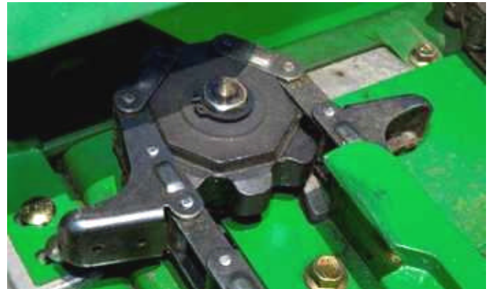
Figure 12- This ADI adjuster sprocket is a durable alternative to steel.
