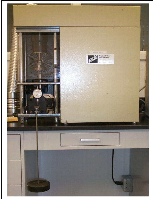
Figure 5: Multi-specimen testing machine
