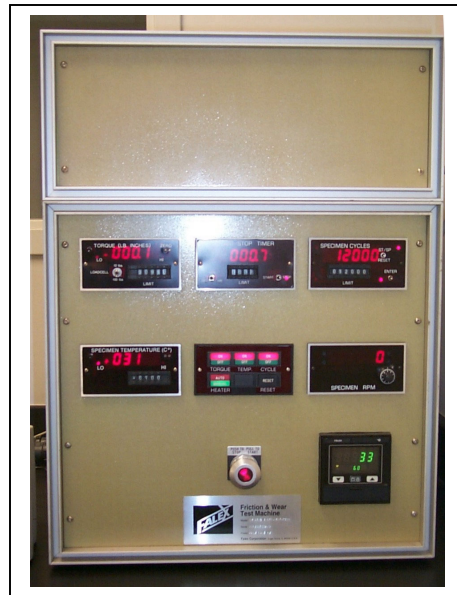
Figure 6: The Control Panel
