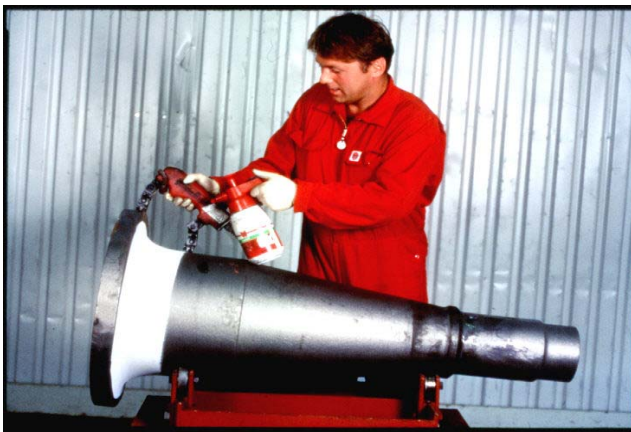
Figure 5 : Ductile Iron Shaft for Wind Mills (390 kg).
